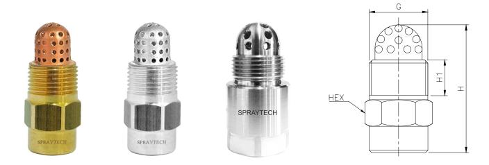
Spraytech's High Velocity Water Spray Nozzles are specially designed for use in fixed water spray or deluge system for the fire protection application. It has internal vane design to generate uniform solid/Full cone spray pattern and dense core of high velocity water spray for efficient fire control.
