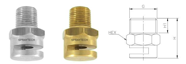
Spraytech' s Curtain Nozzles are sprinklers intended for protection of windows, walls and roofs against exposure fires. It generates uniform flat fan spray pattern and are installed on manual or automatic deluge systems. Window Curtain Nozzles are available in SS and Brass material of construction with different flow rates/K-factors.
