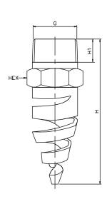
This Spraytech high-efficiency spiral was designed specifically with critical fire and explosion suppression applications in mind. These nozzles feature superior performance unequaled by traditional whirl nozzles.
