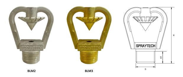
Spraytech Medium Velocity Water Spray Nozzle is an open orifice, directional spray nozzle, designed for use in water spray fixed systems for fire protection applications. They are external deflector-type nozzle that discharge a uniformly filled cone of medium velocity water droplets.
