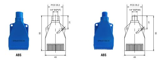
Multi channel flat air spray nozzle have been specially designed for high impact of compressed air with attenuate noise, to obtain an intensive, precise blowing power to minimize cost by reducing air consumption.
